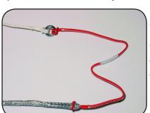
Afterwards loop the 20cm short FDS-Weakpoint-line to the FDS-Endline and then to the 5/10 mm ring.
