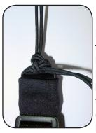
In order to replace the ring, you have to open the bowline knot at the trimmer. You have to use a bowline knot to reconnect the depower leader line to the trimmer. Pull the knot really tight! A short manual at the "support area" on flysurfer.com explains how to make a bowline knot.
